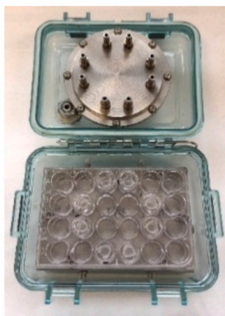
Fig. 1. Exposure box with a standard 24-well plate with 8 active 6-mm inserts.
