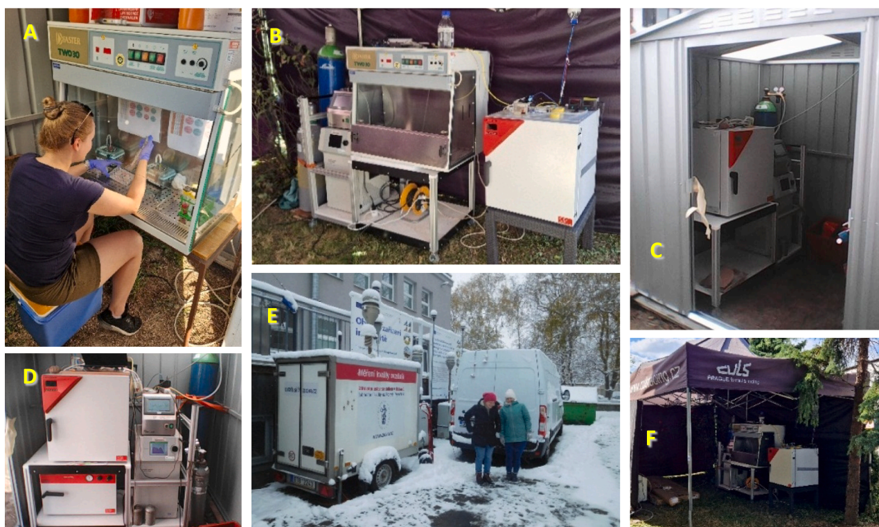
Fig. 3. Field installations of the exposure chamber and the auxiliary laboratory: a,f) laminar flow box placed in a tent; b) left to right: CO 2 and synthetic air bottles, particle counter (UF-CPC 200, Palas) and particle classifier (Engine Exhaust Particle Sizer, TSI), laminar flow box, exposure chamber; c,d) exposure chamber and particle counter and classifier in a 3 m × 2 m lockable garden house; e) winter tests with instruments in a van and air quality monitoring station trailer.
