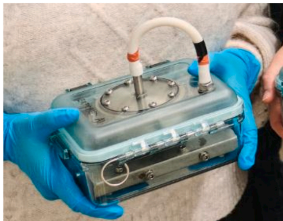
Fig. 1. Exposure box with a standard 24-well plate with 8 active 6-mm inserts.
