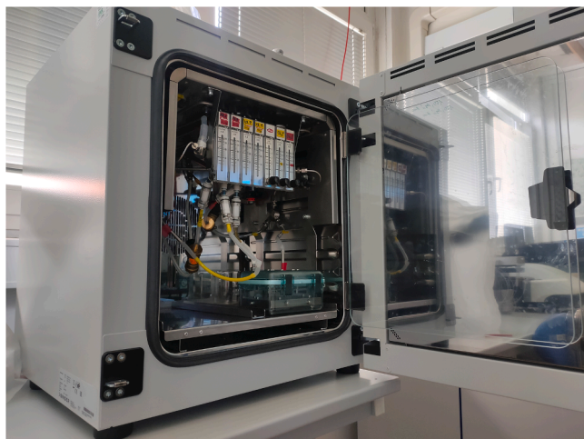
Fig. 2. Development of the exposure system: a commercial incubator housing exposure chambers and other equipment.
